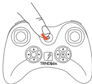
**4.** The controller needs to be calibrated after successful binding: move the throttle/rotate stick to the full up position and then push the throttle/rotate stick to the full down position. When the LED on the controller and the LEDs on the drone are all solid (not blinking), the drone is ready to fly.
